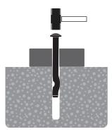
Tap in anchor until seated and flush with surface of fixture.
